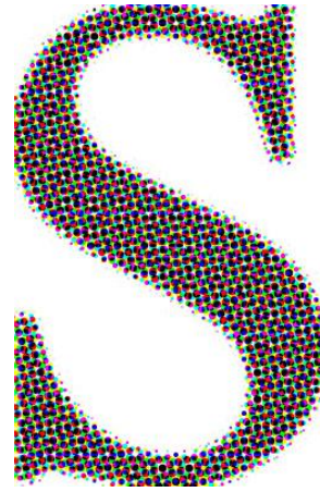
Figure 7: Reproduction of the letter 'S', represented as light projected in dots of red, green and blue.
